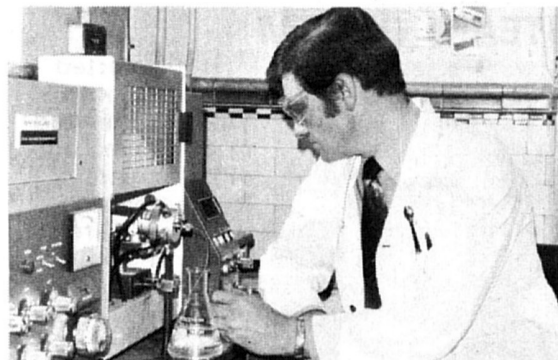
Frank Price at the controls of the atomic absorption spectro-photometer. The machine is easier to use than its name is to pronounce, he says.
