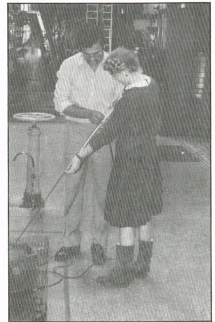
Jay Mistry and Bev Lomas taking water level readings at Somerford Pumping Station during a pumping test. At certain times these measurements had to be repeated several times each minute.
